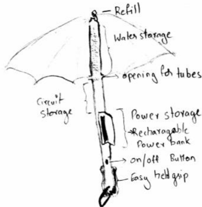
Fig 11. Thumbnail sketch of the humidified umbrella The sketch illustrates the handle with power and water storage
